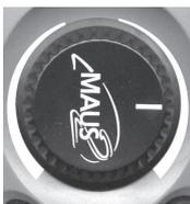
The knob is to control speed and direction of a loco. set to the middle the speed of the loco is 00 and the loco stops. Turning it right you make the loco run forward with increasing speed. Turning the knob to the left the loco runs backwards. Turning it back to the middle makes the loco run slower.
