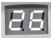
The display, a two digit red LED display tells you the actual selected loco address or selections in menus or their values. It informs you in case of emergency stop, occupied loco addresses or errors. It is easily readable and even in dark rooms visible because it is illuminated.
