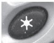
The star-button switches the headlights on and off. Pressing this button the first time the headlights start to shine, pressing it the second time it switches the headlights off. It is important to make sure that the selected speed steps of the loco decoder and the selected speed steps of the Lokmaus®2 will match. If not the headlights don't work correctly or the loco doesn't run (see programming of the CV29 page 25).
