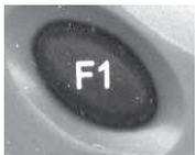
The function buttons 'F1' to 'F4' control the additional functions of a loco such as smoke, digital uncoupler or sound. You also operate the additional functions of a car equipped with a function decoder e. g. headlights, illumination or signal horn. Pressing this button the first time it switches on the function, pressing it a second time it switches off the function.
