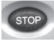
The button 'stop' causes an emergency stop. All locomotives stop and the feeding of the layout is interrupted. During this emergency stop mode you can select new loco addresses and give commands to those locos e.g. to stop them or give new commands so that they don't continue their way after releasing the stop-mode. Pressing 'STOP' the second time you release the stop mode and the locos re-start to run. The commands you gave during the stop-mode are executed now immediately.
